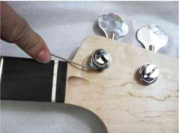
Ensure that the string sits smoothly on its saddle and keep taut whilst winding a couple of turns on the relevant tuner. Thread through the string post and bend the string back on itself to anchor it in place. Apply a little tension from the tuner and move on to the next string. Repeat the above process for all four strings.
