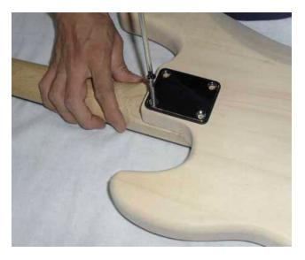
Turn the assembly over and position the neck plate (with its black protective seal) over the four bolt holes at the rear of the body and drive in the four long screws through the neck plate, body and pilot holes in the neck until all fits tightly.
