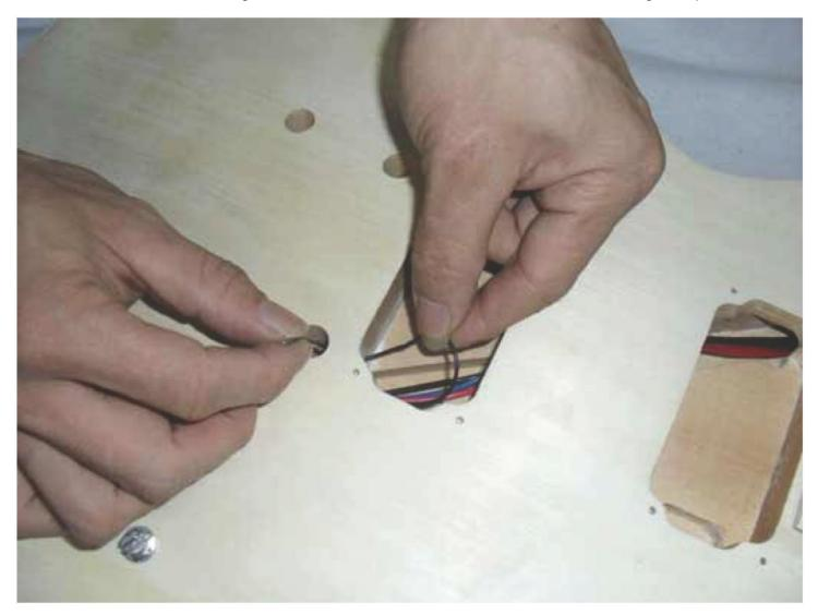
Lead the cables of the pickups from the pickup cavity through the channel to the control cavity and connect them to the potentiometers accordingly.
