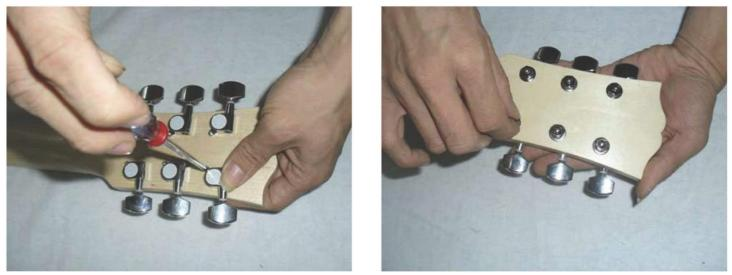
Tighten the nut on the front face of the tuner until it is firm by using a spanner of the correct size. Repeat this for the remaining five tuners.
