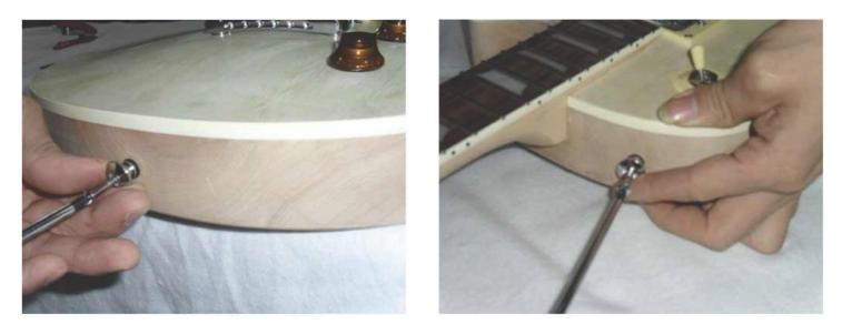
Screw the strap buttons into the pre-drilled holes at the bottom edge of the body and at the top next to the switch.
