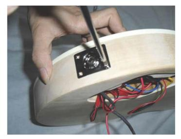
Connect the switch with the three cables coming from the control cavity according to the marking numbers located on the connectors. Put the switch on the right position and fix it from the front side.
