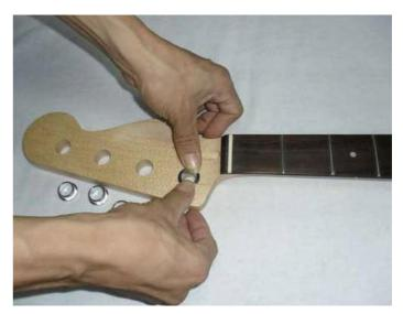
Fix the retaining screw through the loop on the rear of the gear housing into the pilot hole to hold the tuner in position. Tighten the nut on the front face of the tuner until it is firm by using a spanner of the correct size. Repeat this for the remaining three tuners and then fit the string tree.
