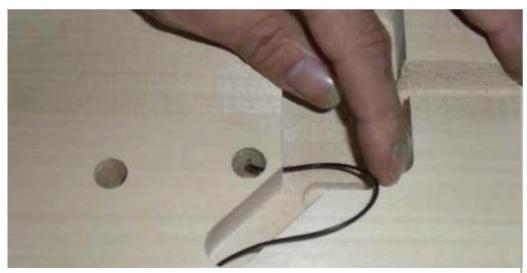
Lead the cables of the pickups from the pickup cavity through the channel to the control cavity and connect them to the potentiometers accordingly.
