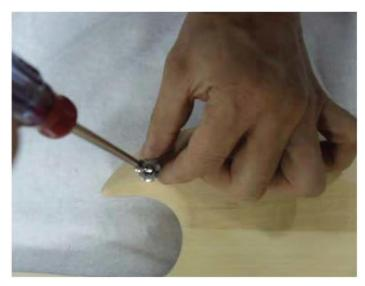
Screw the strap buttons into the pre-drilled holes at the bottom edge of the body and at the rear of the upper horn.
