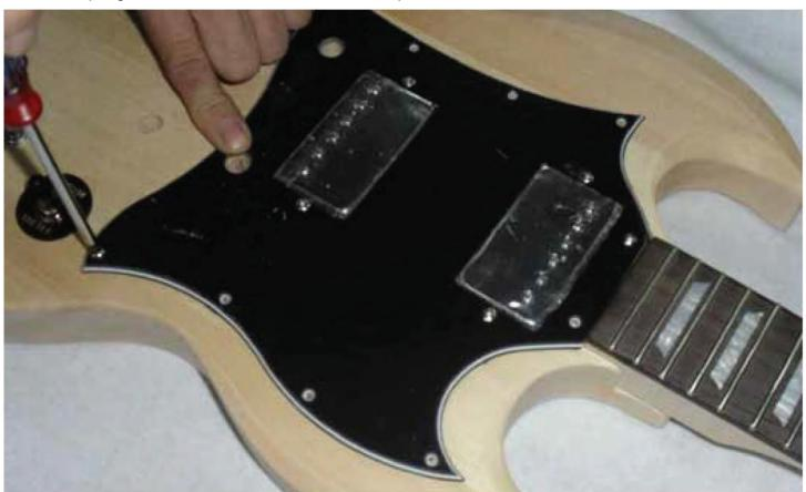
The rear body plastic plate now can be fitted to cover the control and switch cavity. Secure the plate with dome-head screws into the pre-drilled holes.
