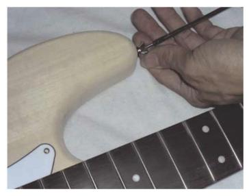
Screw the strap buttons into the pre-drilled holes at the bottom edge of the body and at the tip of the upper horn of the body.
