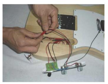
Gently thread the cable on the potentiometers lead through the hole behind the tone control cavity to the separate routing for the jack socket. Connect the connector wire to the connector on the jack socket (they only fit one way round), then fit the jack socket plate and secure it with dome-head screws.
