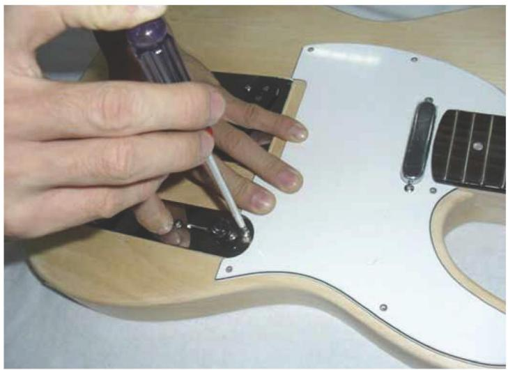
Now position the pickguard, bridge, and control panel on the front of the body in a way that the pickups and all the wiring sit neatly in the routed cavities. Ensure that the edge of the pickguard sits snugly at the end of the neck and straight to the bridge assembly. Secure the pickguard with the small dome-head screws provided into the pre-drilled pilot holes.
