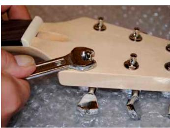
Tighten the nut on the front face of the tuner until it is firm by using a spanner of the correct size. Repeat this for the remaining five tuners.
