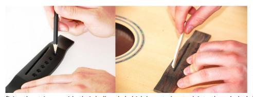
Sequencing all the pre drilled holes on the surface of the bridge have to be drilled carefully and completely through the top (1<sup>st</sup> photo on the left side). The diameter of each hole should be not wider than 0,6mm to 0,7mm!!! If you use a wood drill with a bigger size it can occur that the bridge pins for
