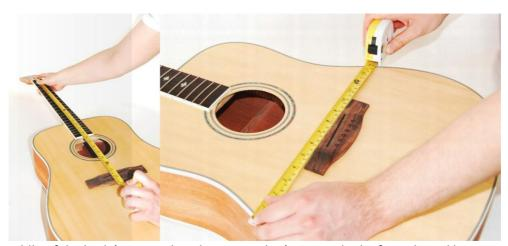
must be placed exactly in the middle of the body's top so that the strings don't run aside the fingerboard later. Check the 2<sup>nd</sup> photo above on the right. At all: Before fixing the bridge you should survey the exact position of it - marking that with a lead pencil.
