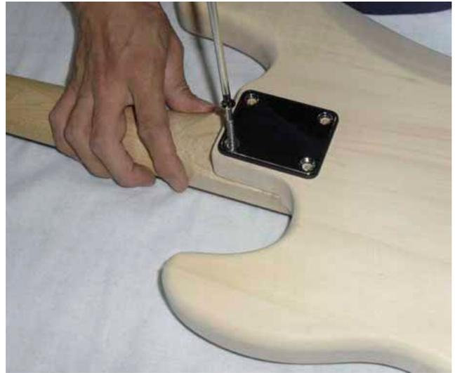
Turn the assembly over and position the neck plate (with its black protective seal) over the four bolt holes at the rear of the body and drive in the four long screws through the neck plate, body and pilot holes in the neck until all fits tightly.
