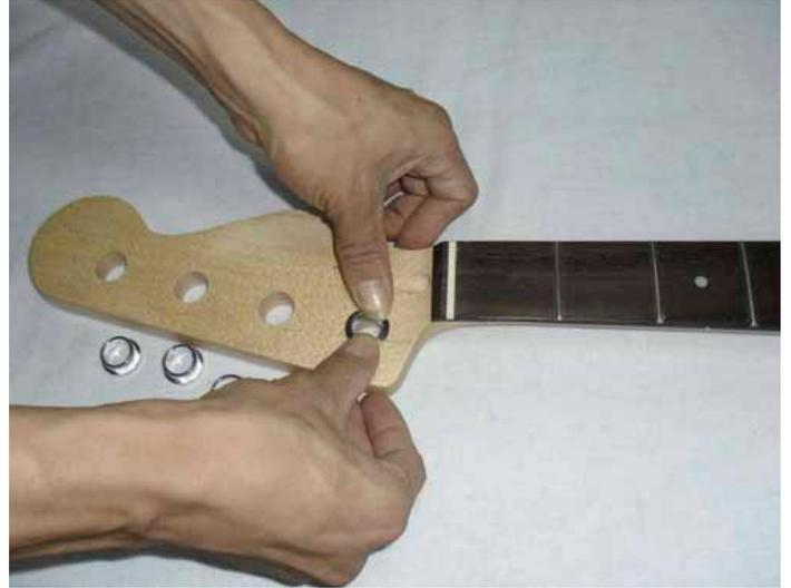
Fix the retaining screw through the loop on the rear of the gear housing into the pilot hole to hold the tuner in position. Tighten the nut on the front face of the tuner until it is firm by using a spanner of the correct size. Repeat this for the remaining three tuners and then fit the string tree.
