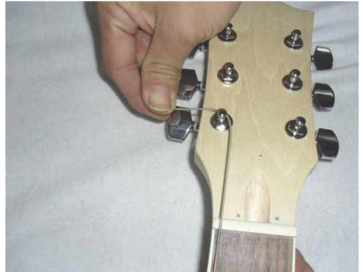
Ensure that the string sits smoothly on its saddle and keep taut whilst winding a couple of turns on the relevant tuner. Thread through the string post and bend the string back on itself to anchor it in place. Apply a little tension from the tuner and move on to the next string. Repeat the above process for all six strings.
