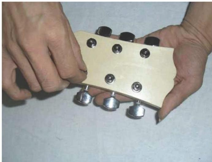
Tighten the nut on the front face of the tuner until it is firm by using a spanner of the correct size. Repeat this for the remaining five tuners.
