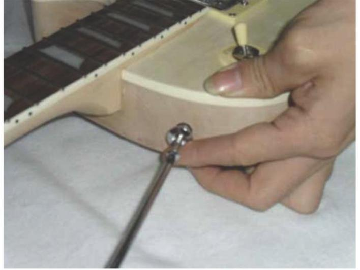
Screw the strap buttons into the pre-drilled holes at the bottom edge of the body and at the top next to the switch.
