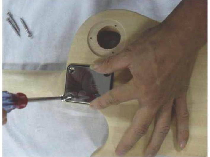
Turn the assembly over and position the neck plate (with its black protective seal) over the four bolt holes at the rear of the body and drive in the four long screws through the neck plate, body and pilot holes in the neck until all fits tightly.
