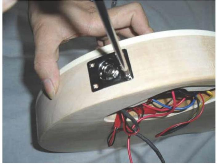
Connect the switch with the three cables coming from the control cavity according to the marking numbers located on the connectors. Put the switch on the right position and fix it from the front side.
