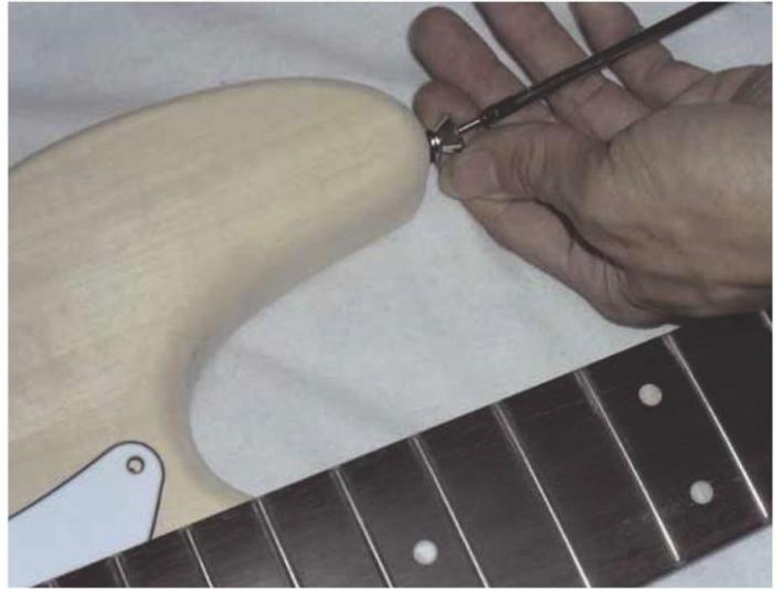
Screw the strap buttons into the pre-drilled holes at the bottom edge of the body and at the tip of the upper horn of the body.
