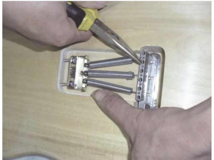
Turn the guitar over and screw the spring claw part-way into the pre-drilled holes at the forward edge of the rear body cavity
