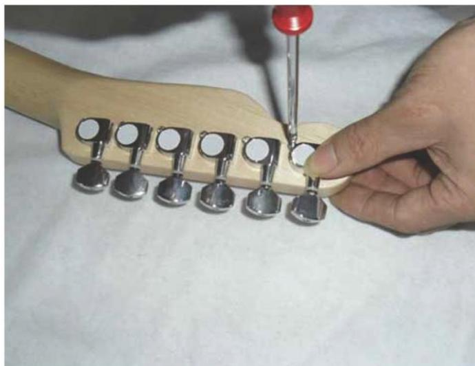
Fix the retaining screw through the loop on the rear of the gear housing into the pilot hole to hold the tuner in position. Then tighten the nut on the front face of the tuner until it is firm by using a spanner of the correct size. Repeat this for the remaining five tuners and then fit the string tree.
