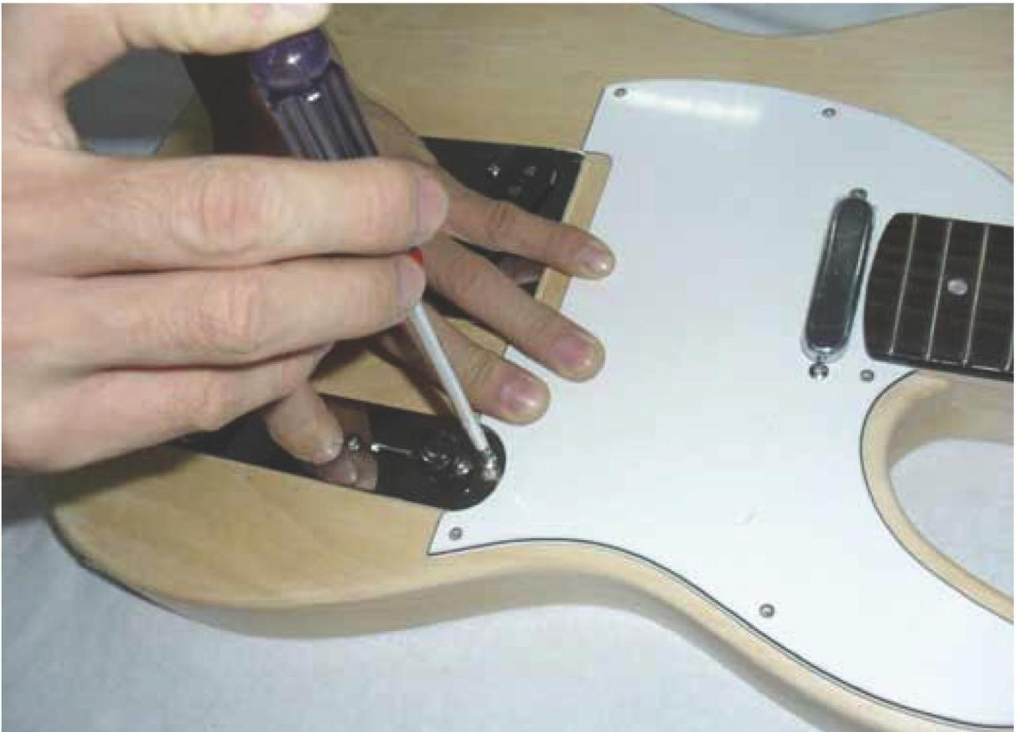
Now position the pickguard, bridge, and control panel on the front of the body in a way that the pickups and all the wiring sit neatly in the routed cavities. Ensure that the edge of the pickguard sits snugly at the end of the neck and straight to the bridge assembly. Secure the pickguard with the small dome-head screws provided into the pre-drilled pilot holes.
